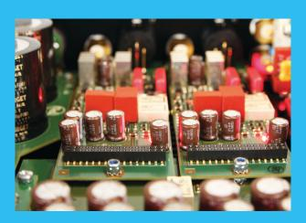
The Primary amplification is performed in the transistor input stage by our double mono construction, fitted with double FET inputs. With no error current, these provide unlimited input resistance, and under conditions of minimal constant capacity have an almost unlimited input resistance.
