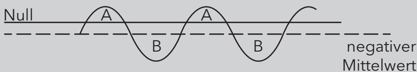
Mean value of an unbalanced AC voltage supply (DC component)
