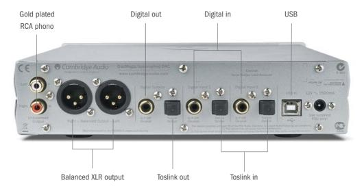
With a variety of simple connections including S/PDIF, Toslink and USB inputs, DacMagic can be set-up in seconds. Key to its abilities is Adapted Time Filtering (ATF™) upsampling technology and twin Wolfson DACs which provide outstanding stereo imaging.
