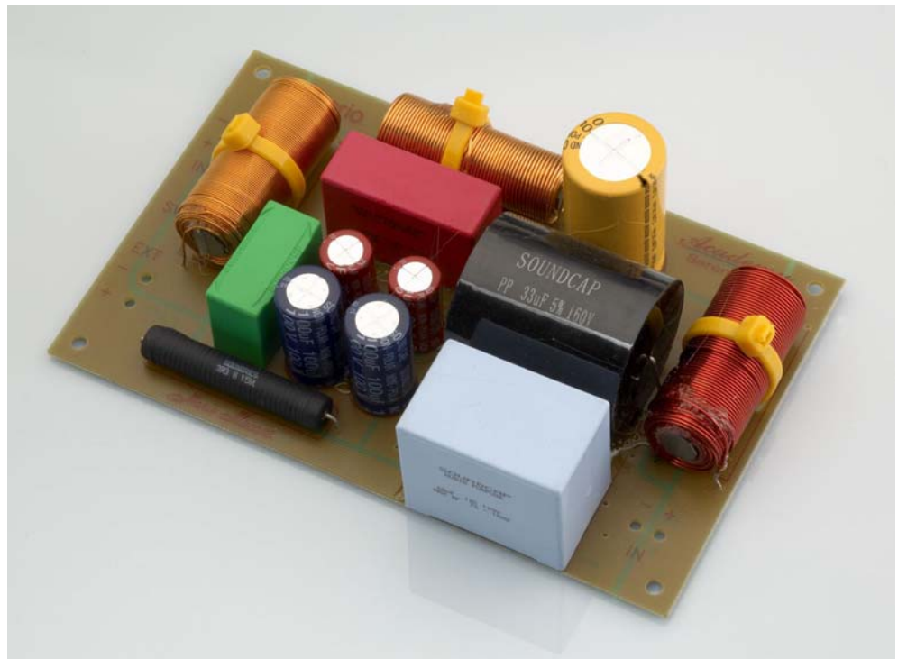
Subwoofer Crossover – Nuclei IRON POWDER & Induttori HIGH Q
