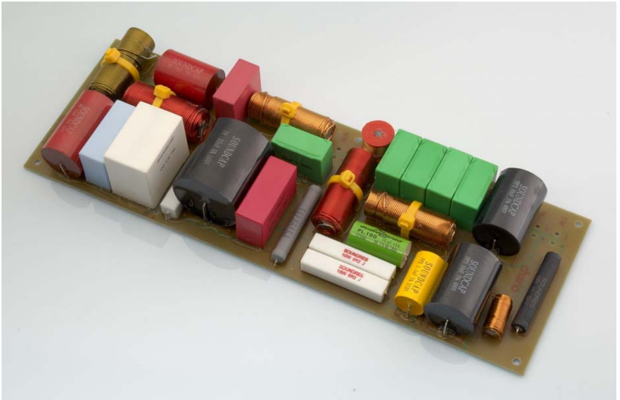
Medio-Akti Crossover – SOUND CAP™ High Grade & Resistori MIL
