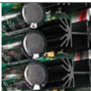
DC regulation for the analog supply is located near the front channel outputs on the right side of the chassis.
