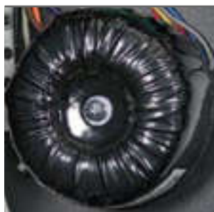
A custom designed low-noise toroidal transformer is used for the analog circuitry's linear power supply.
