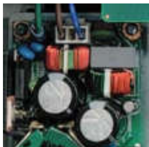
An independent low-voltage, high-current supply powers digital circuits.
