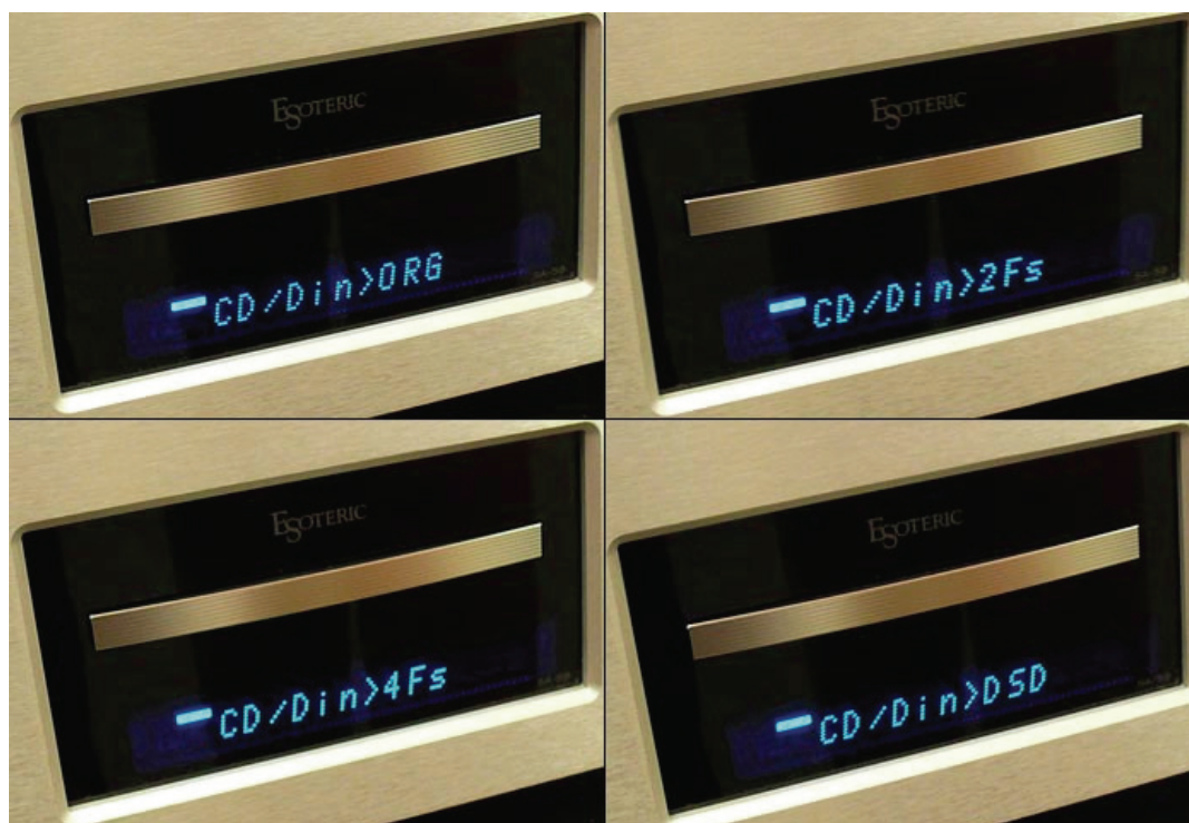
Conversion settings for CD or "digital inputs," shown in the above photos (CD/Din). Photos courtesy of www.6moons.com
