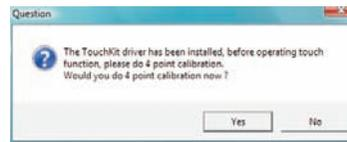
8 Click 'Yes' to perform a 4 point calibration. This is required for proper touch screen operation.
