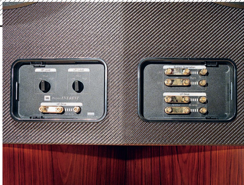
ABOVE: Cover plate on the baffle conceals switches for tweaking HF/LF levels, and links to hand the speaker and disable the network for active drive
