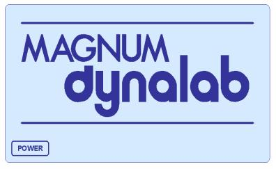
9. To turn on the unit push the power button. At first the screen will display "warming up" as the components are brought up to a safe operating condition. Once the safe operating condition is attained, the screen that is associated with the setting of the input knob will appear. If you are using it in the FM tuner mode, FM will appear on the left side of the screen.
