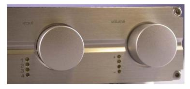
**Input Selection Knob** (left knob) – Push it in to turn P-8 On and Off. Turn the knob to select Input 1, 2, 3, or 4. If the P-8 is muted, pushing the Input Selection Knob once will bring P-8 out of muting.
