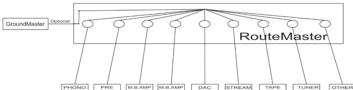
RouteMaster accepts grounding reference connections from up to nine system components. Simply identify a spare input and connect it with the appropriate Ultra Connect cable. For the very optimum results all RouteMaster UltraConnects should be the same length and hence resistance.
