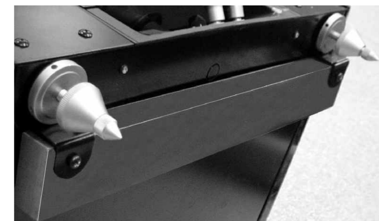
B Attaching the stabiliser and rear feet
