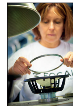
New Sopra midrange drivers being assembled at our Ariane manufacturing facility. This facility based on lean manufacturing employs highly-qualified workers who have complete control over every step of the process.
