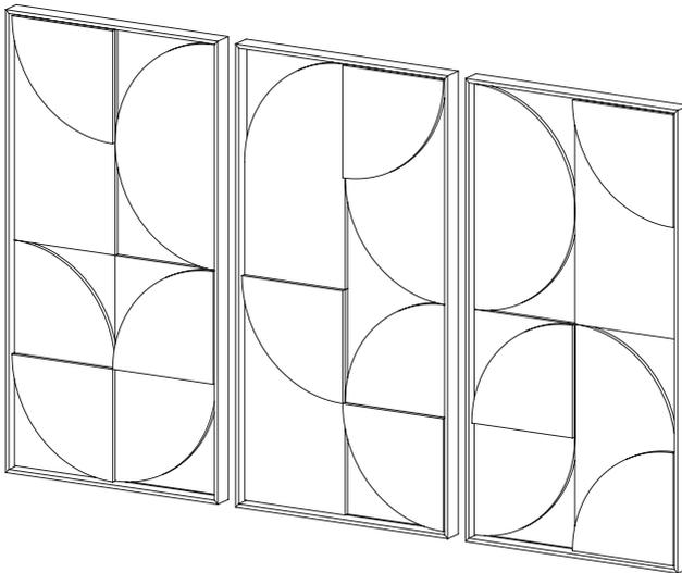
If you choose to install the panel horizontally, unscrew the suspension clip and screw it into the middle of the long side of the frame (580mm from the edge).
