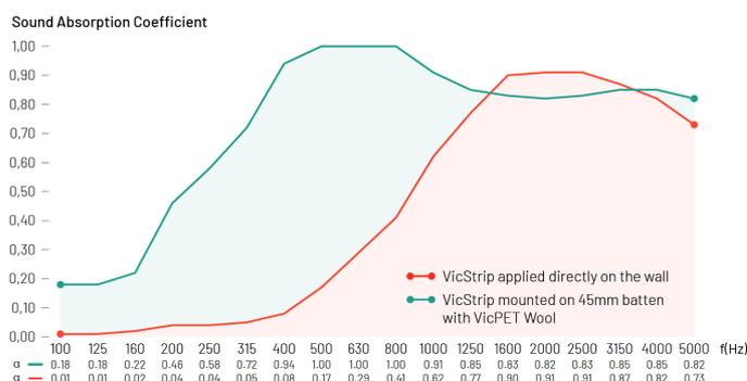
NRC: VicStrip applied directly on the wall: 0.45; VicStrip mounted on 45mm batten with VicPET Wool (40mm) behind the panels: 0.85.
